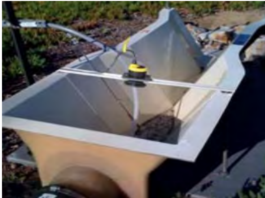
Numerous commercial water level/telemetry systems are available to measure flow remotely, including ultra-sonic and other sensors.
