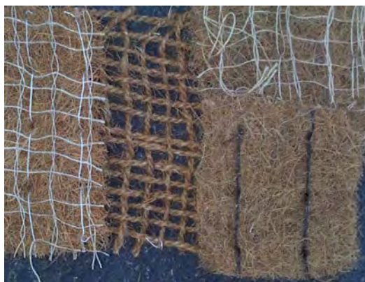
Natural fiber erosion fabrics are commonly made with coconut or jute.
