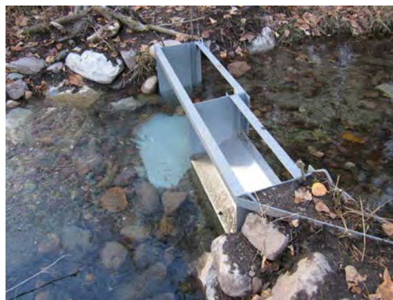
In a Coanda, water flows down and out of a pipe, while fish and debris pass over the screen.
