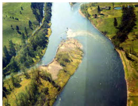
Berms can direct flow against the opposite bank and cause erosion on the other side of the river.
