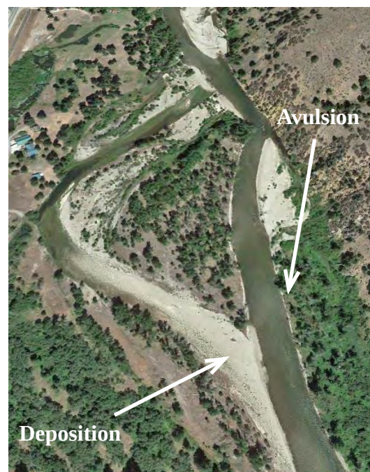
Bitterroot River channel cutoff in 2014. Sediment has deposited on the left meander channel. Note rip-rap in left channel to protect home.
